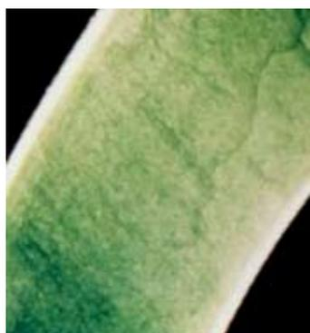
Fig. 5. B+C-jade bangle, note the colour concentration along fissures and between grain boundary viewed under transmitted lighting (20x). © Tay Thye Sun
