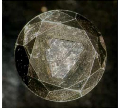
Fig 2: Black diamond with colourless central zone and black rim due to many small black inclusions. © H.A. Hänni, SSEF 2005
