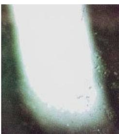
Fig. 2. Mirror-like surface reflection of a natural untreated jadeite-jade viewed under reflected light (20x).
