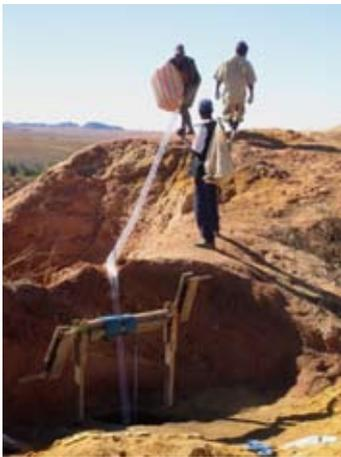
Fig. 3: While a man works at the bottom of the 18m shaft his partners keep the oxygen flowing. © C. Verny-White, 2006
